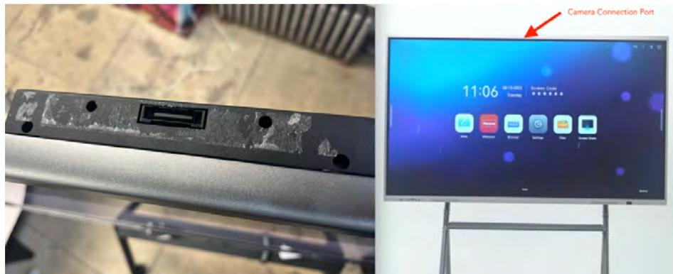
2. Mount the camera by lining up the 2 guide pins and gently pressing down until the modular connector is properly seated.
